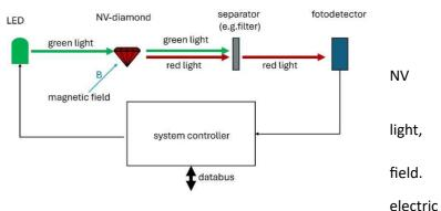
Magnetic fields, temperature, fields, or mechanical parameters are determined with high sensitivity from this signal.
